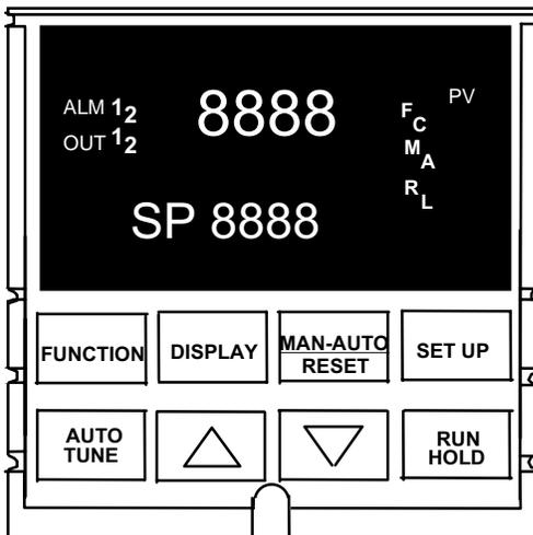
Figure 1-1 ETC023 Operator Interface
