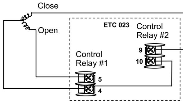
Figure 2-9 3-Position Step Control Connections for Internally Powered Motors
