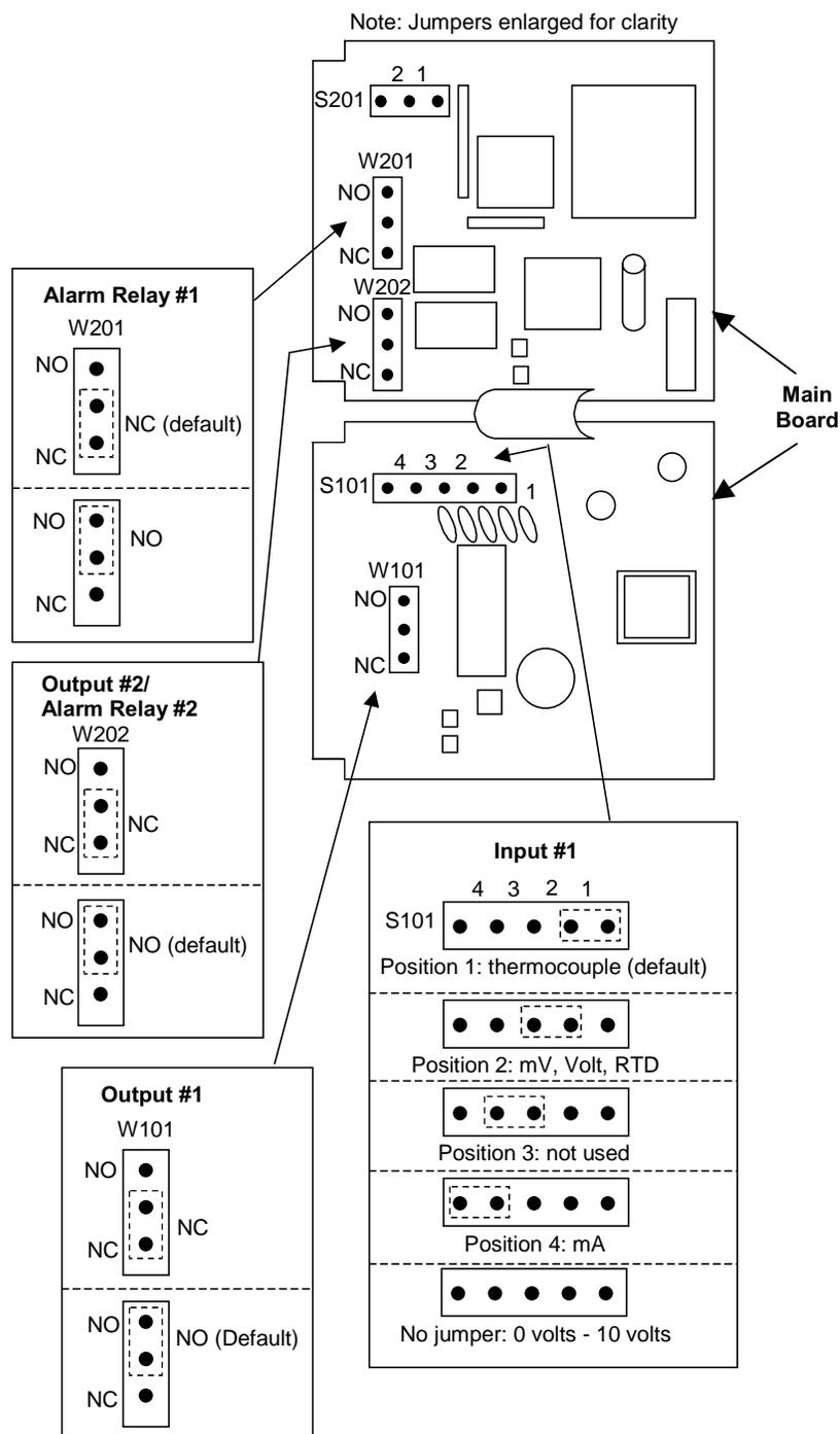
Figure 2-1 Jumper Placements
