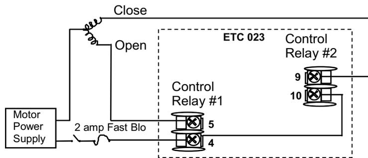
Figure 2-10 3-Position Step Control Connections for Externally Powered Motors
