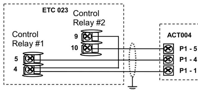
Figure 2-11 3-Position Step Connections for Eclipse Rotary Actuator
