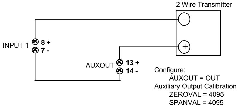
**Figure 2-14 Transmitter Power for 4-20 mA - 2 Wire Transmitter Using Auxiliary Output**
