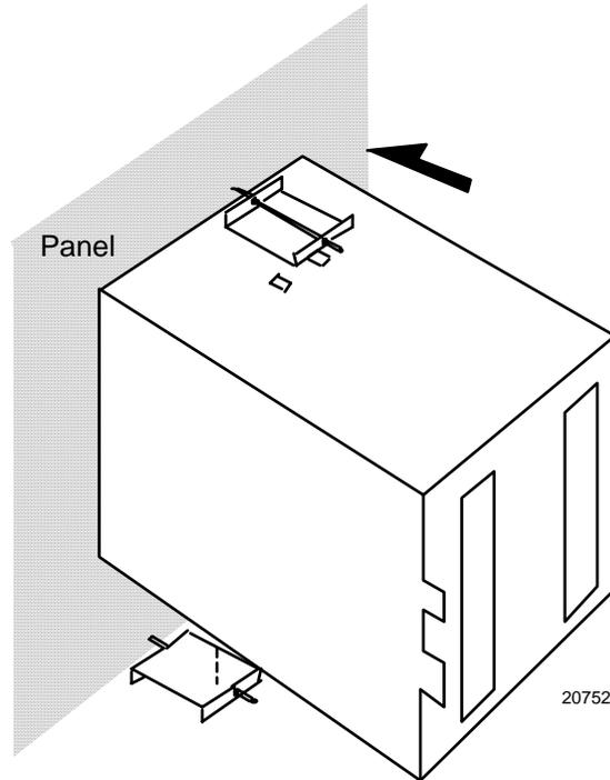
Figure 2-3 Mounting Method
