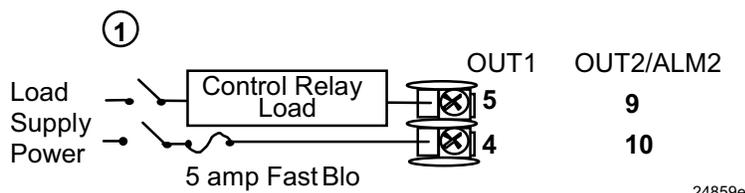
① Control relays are configured N.O. as shipped. Alarm relays are configured N.C. as shipped. N.O. or N.C. configurations are selectable by jumpers on the main printed wiring boards.
