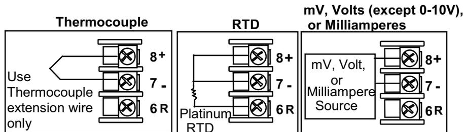
**Figure 2-6 Input 1 Connections**
